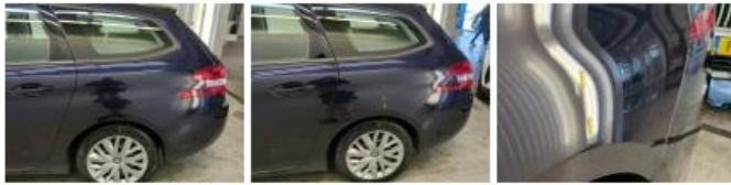
Wing FL, Scratch(es), Repair and paint (complete)
