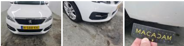
Bumper F, Scratch(es), Repair and paint (partial)
