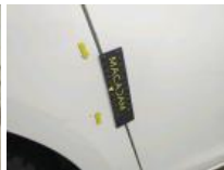
Boot lid covering R, Scratch(es), Replace
