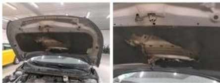
Engine insulation, Damaged, Replace
