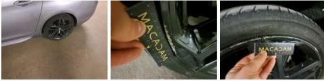
Boot cover, Missing, Replace
