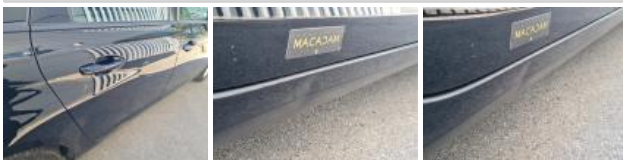
Outer sill R, Dent(s), Spot repair
