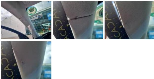
Roof liner, Burned, Smart repair
