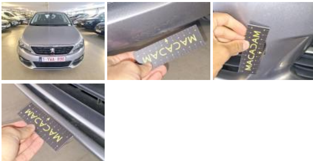
Bonnet, Bad repair, Repair and paint (complete)
