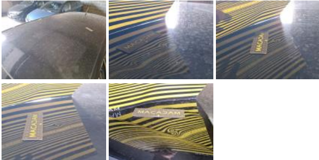
Roof, Hail damage, Forfeit hail (heavy)
