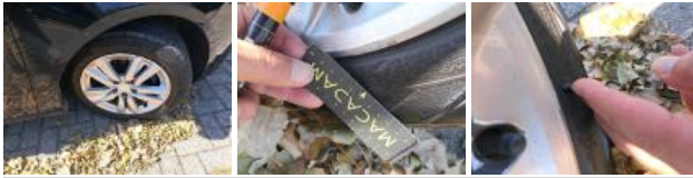
Tyre RR, Tear, Replace
