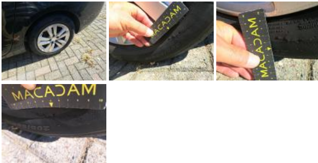
Tyre FL, Tear, Replace
