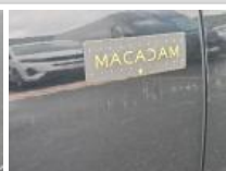
Door FR, Scratch(es), Repair and paint (complete)
