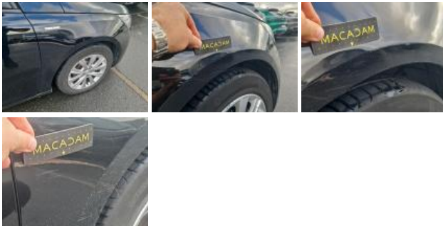
Tyre FR, Tear, Replace
