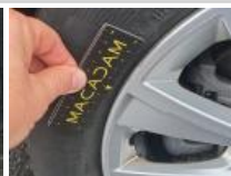
Tyre RR, Tear, Replace
