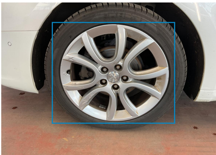
7. Rim / Front Left Out of Bodywork / Scratch -
