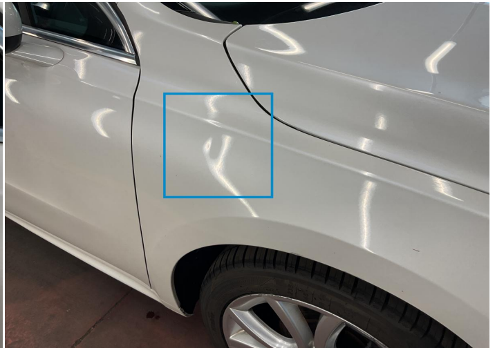
20. Fender / Front Right Bodywork / Dent -
