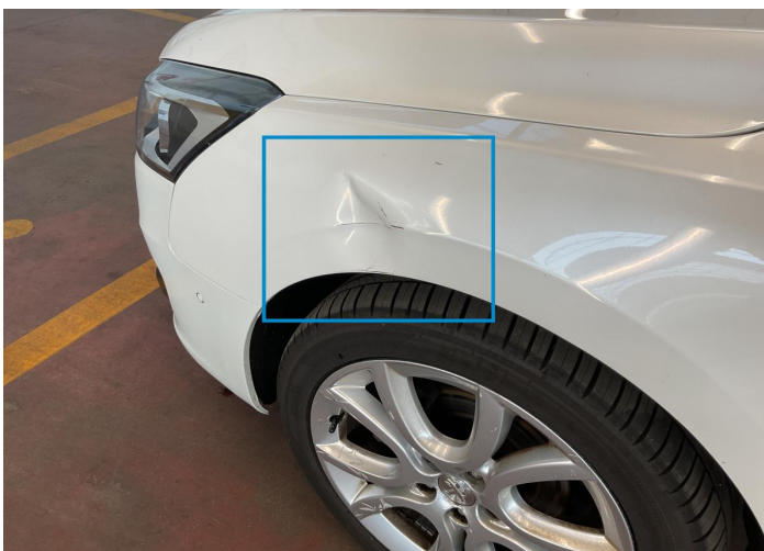
8. Fender / Front Left Bodywork / Dent -
