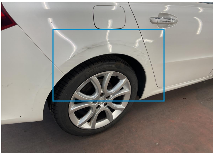
15. Fender / Back Right Bodywork / Dent -
