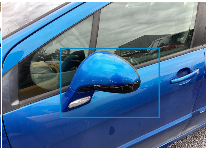
18. Mirror / Front Left Bodywork / Breakage -
