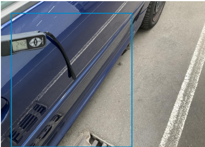
5. Door / Front Right Paint / Poor Previous Repair -
