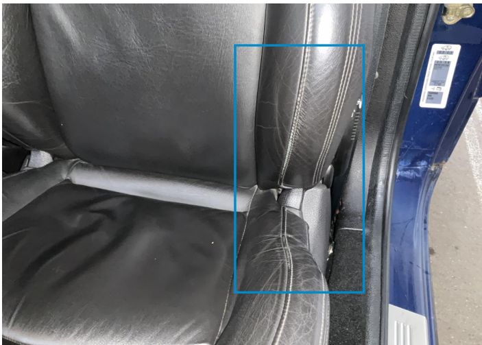
1. Seat / Front Left Interior / Worn - out -
