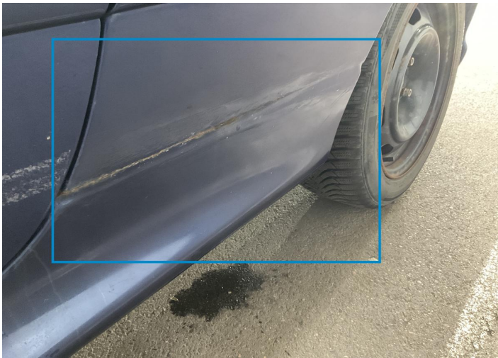
11. Side Panel / Back Left Paint / Corrosion -
