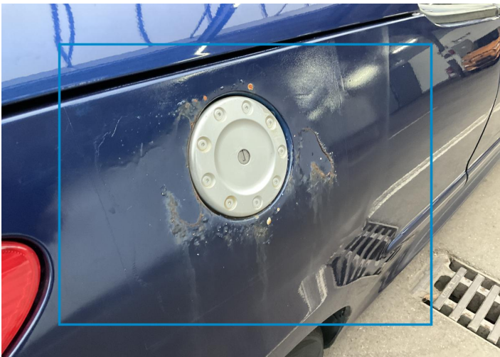
8. Side Panel / Back Right Paint / Corrosion -
