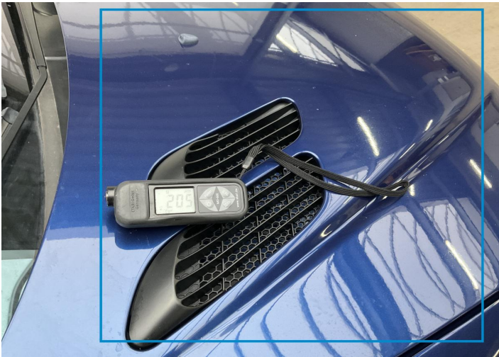
4. Hood Paint / Poor Previous Repair -
