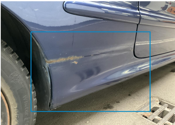
7. Side Panel / Back Right Paint / Corrosion -
