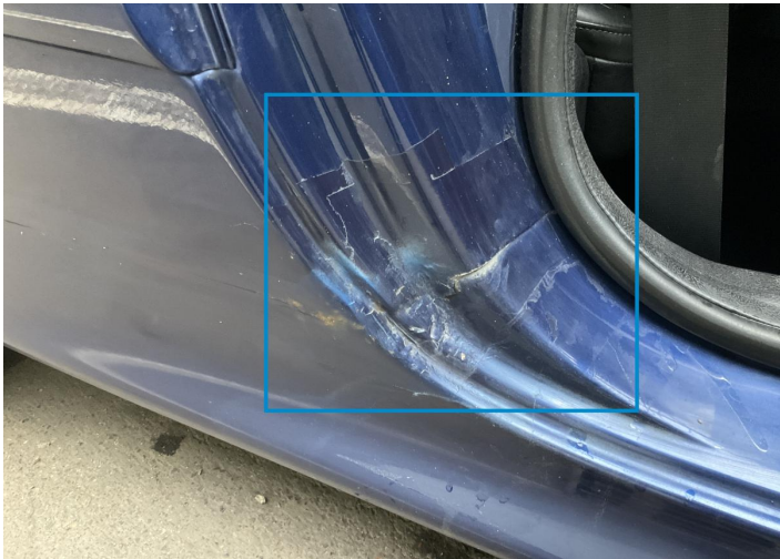
3. Rocker Panel / Center Right Paint / Poor Previous Repair -
