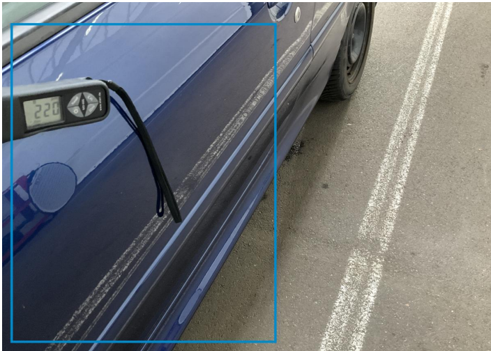
10. Door / Front Left Paint / Poor Previous Repair -
