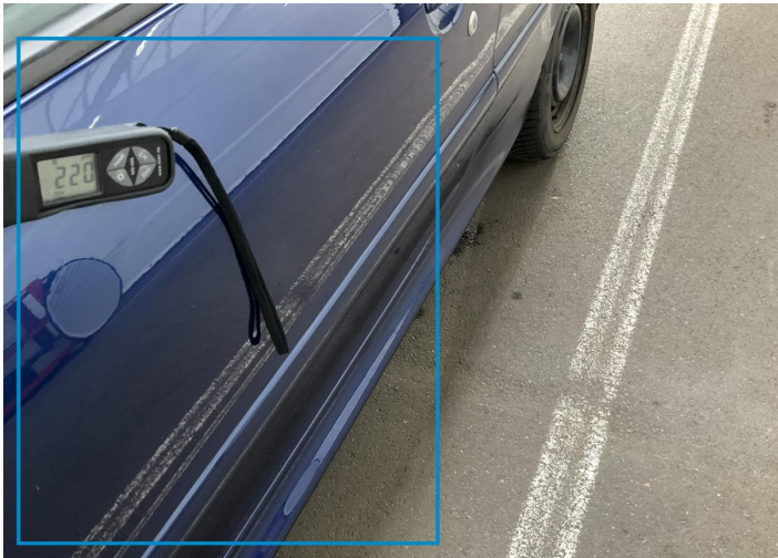
10. Door / Front Left Paint / Poor Previous Repair -
