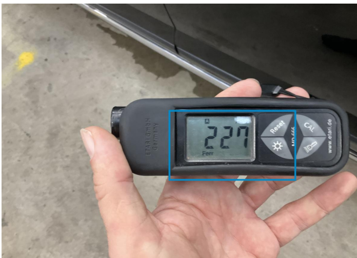
16. Door / Back Left Paint / Poor Previous Repair -
