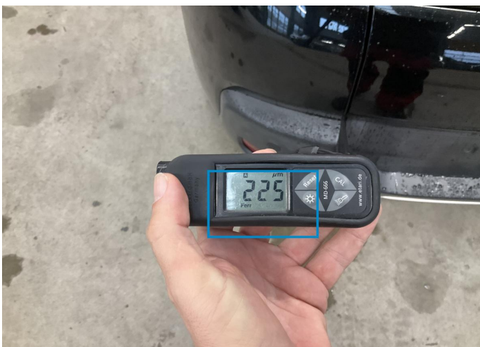
14. Tailgate Paint / Poor Previous Repair -
