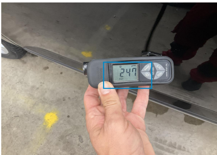
17. Door / Front Left Paint / Poor Previous Repair -
