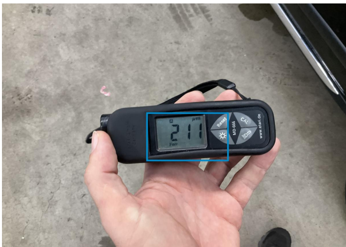
15. Fender / Back Left Paint / Poor Previous Repair -
