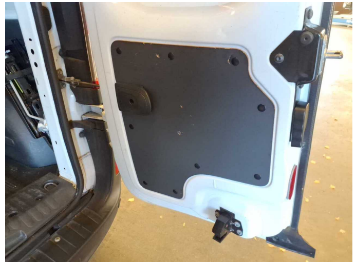
Damage 7: Trim / covers: Boot lid - interior trim (Rechts) - Broken / torn - Replace
