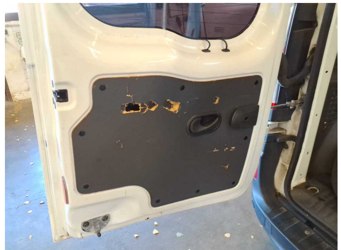
Damage 8: Trim / covers: Boot lid - interior trim (Links) - Broken / torn - Replace
