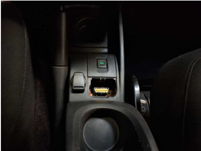
Damage 1: Instrument panel: Centre console - front (Abdeckung OBD Stecker) - Missing - Replace
