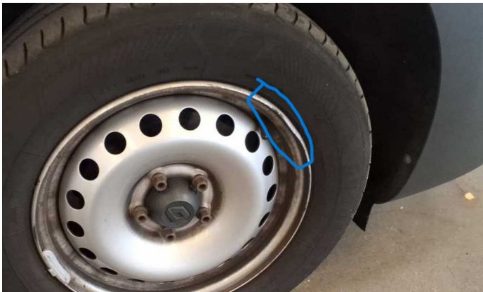
Damage 2: Wheel / tyres: Wheel rim - front right side - Damaged - Replace
