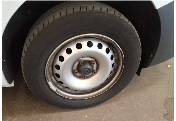
Damage 2: Wheel / tyres: Wheel rim - front right side - Damaged - Replace
