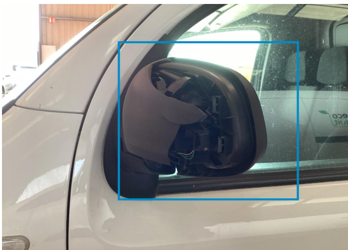
5. Mirror Shell / Front Left Bodywork / Breakage -
