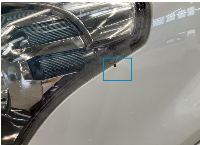
4. Fender / Front Left Paint / Corrosion -
