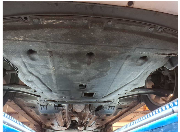
Damage 1: Engine: Engine cowl - lower - Holes - Replace
