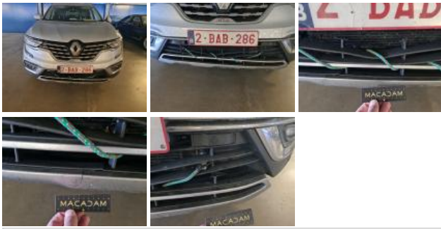
Bumper moulding F, Broken, Replace
