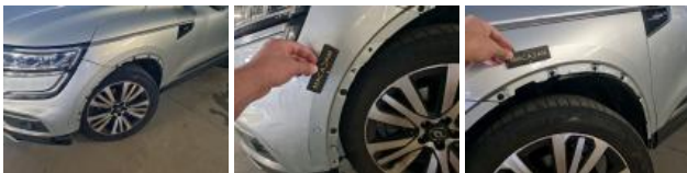
Wheel arch cover FL, Missing, Replace
