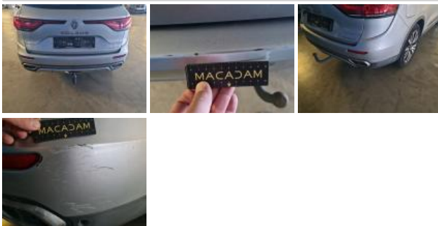
Bumper moulding R, Scratch(es), Replace
