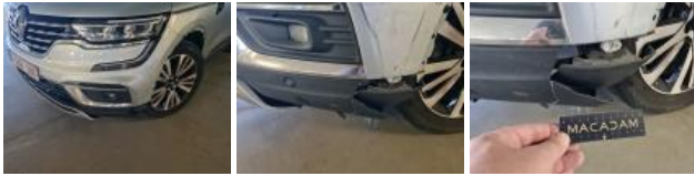
Bumper F, Broken, Replace and paint
