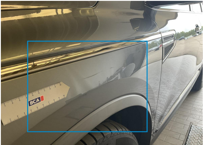
1. Fender / Front Left Paint / Scratch / Scuff -
