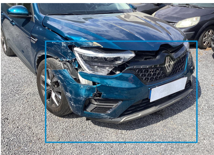
4. Bumper / Front Bodywork / Dent / Deformation -
