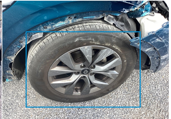
20. Rim / Front Right Out of Bodywork / Breakage -
