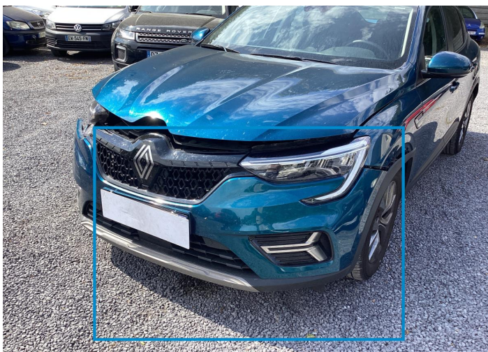
5. Bumper / Front Bodywork / Dent / Deformation -
