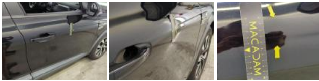
Door RR, Scratch(es), Repair and paint (complete)
