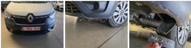
Wing trim FL, Missing, Replace
