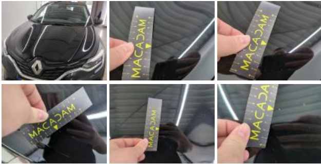
Bumper F, Scratch(es), Repair and paint (complete)
