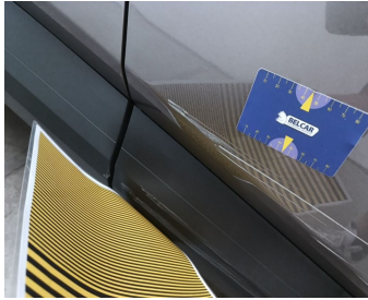
Door Front Right // Repair & Painting-scratch + dent
