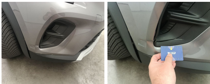
Bumper Front / Grid Right / Replace-tear
