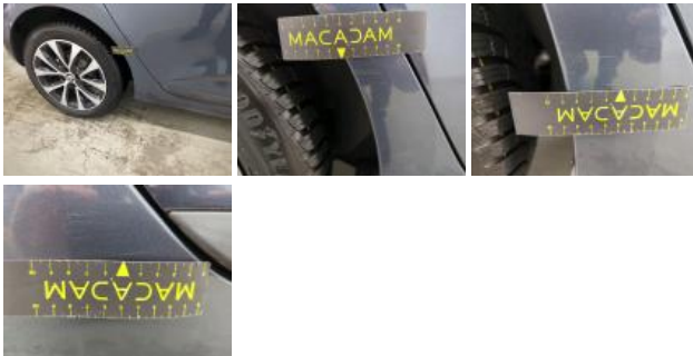
Door FR, Scratch(es), Repair and paint (complete)
