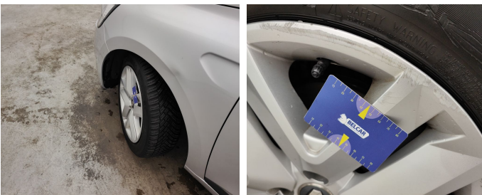
Wheel Front Left / Wheel Cover / Replace-scratch
