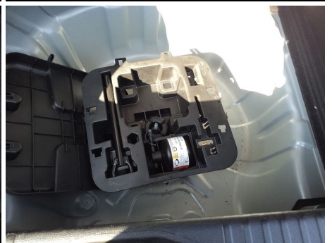
Compressor tyre repair kit / - / Missing
