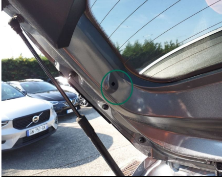
Rear parcel shelf retaining strap hook / Back Left / Missing
