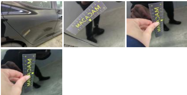
Door FR, Scratch(es), Repair and paint (complete)
