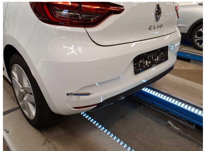
Damage 6: Rear bumper: Rear bumper - Scratch(es) - Paint
