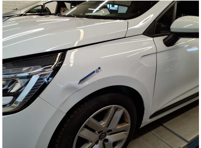
Damage 7: Mudguard - left side: Mudguard - left side - Deformed - Repair and paint
