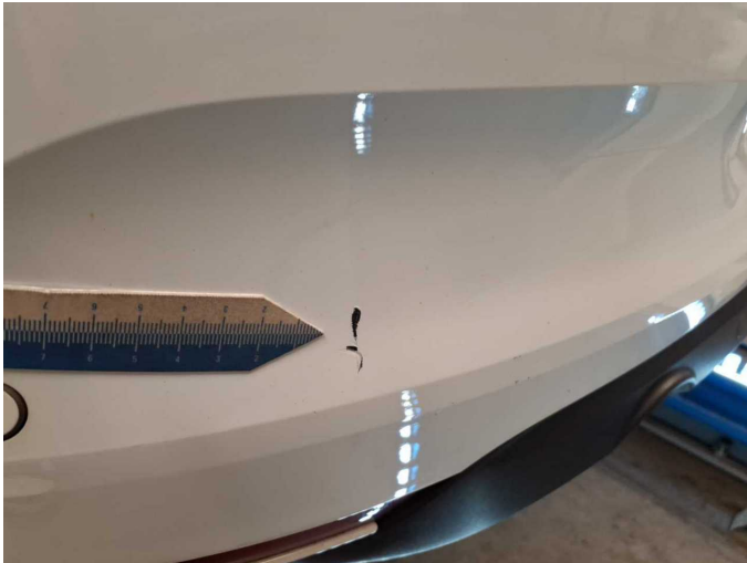
Damage 6: Rear bumper: Rear bumper - Scratch(es) - Paint
