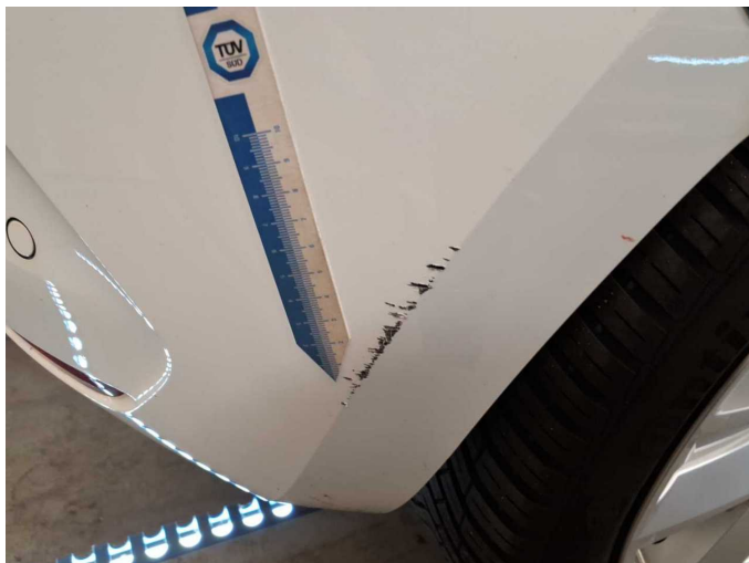
Damage 6: Rear bumper: Rear bumper - Scratch(es) - Paint
