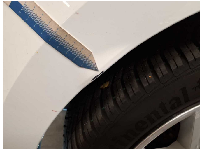
Damage 6: Rear bumper: Rear bumper - Scratch(es) - Paint
