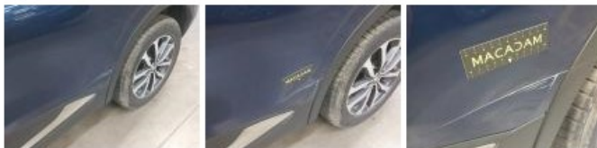
Wing trim RL, Scratch(es), Replace
