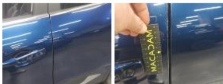
Door RL, Dent(s) and scratch(es), Spot repair
