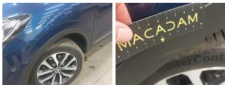
Door FL, Scratch(es), Spot repair
