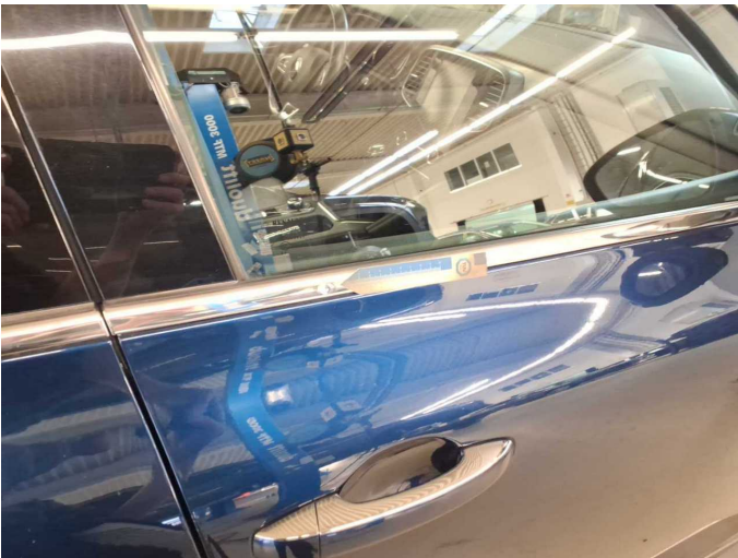
Damage 1: Door - front right side: Strip - outer - Deformed - Replace
