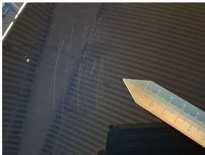
Damage 7: Bonnet: Bonnet (+ Kratzer) - Paint defect - Paint
