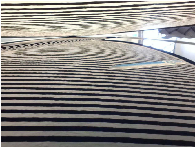
Damage 10: Roof: Roof (+ Lackmängel) - dent(s) - Repair and paint
