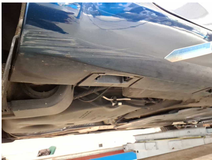
Damage 2: Sill - right side: Trim - Scratched - Repair and paint
