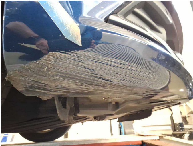
Damage 11: Front bumper: Bumper with Parktronic (+ verschürft) - Deformed - Replace
