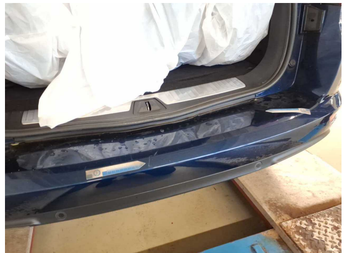
Damage 5: Rear bumper: Bumper with Parktronic - Scratch(es) - Paint
