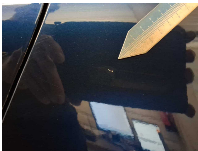
Damage 3: Side panel - rear left side: Side panel - Dent / paintcoat damage - Smart repair
