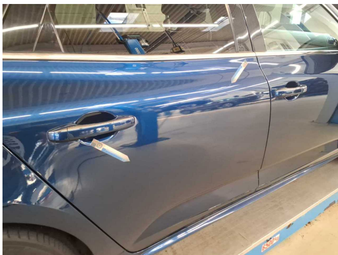
Damage 9: Door - rear right side: Door (wellig + Folgeschaden) - Unprofessionally repaired - Repair and paint
