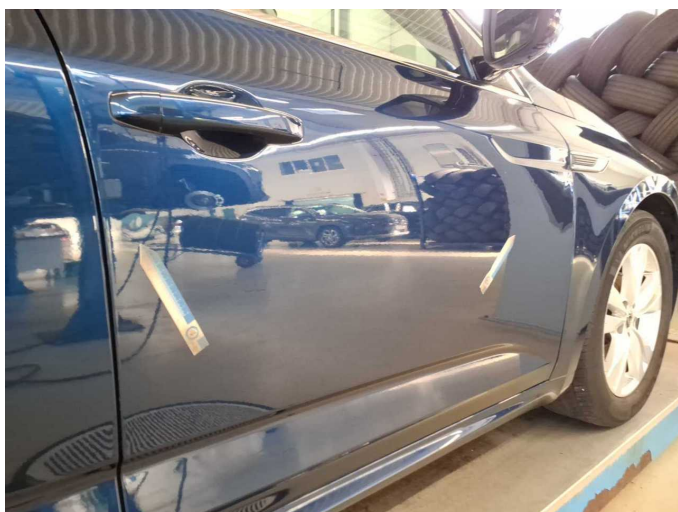
Damage 8: Door - front right side: Door (wellig + Folgeschaden) - Unprofessionally repaired - Repair and paint
