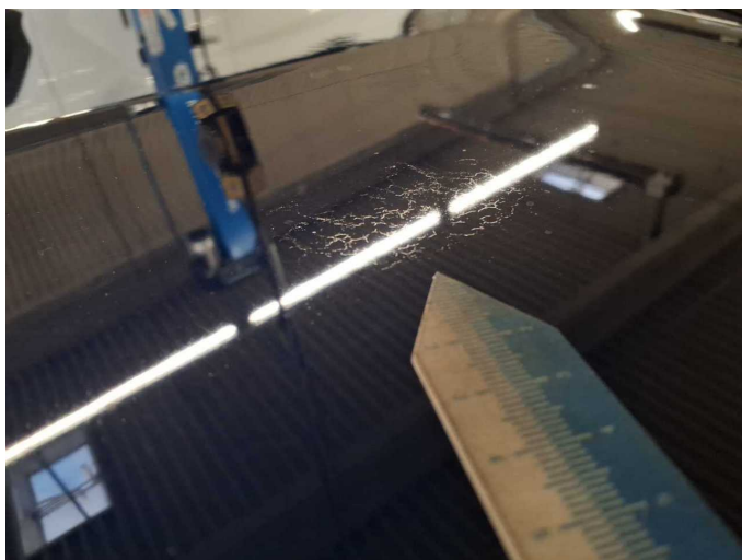
Damage 7: Bonnet: Bonnet (+ Kratzer) - Paint defect - Paint
