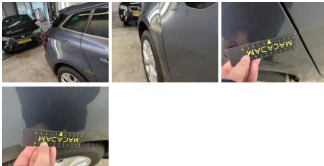
Door FR, Scratch(es), Repair and paint (complete)
