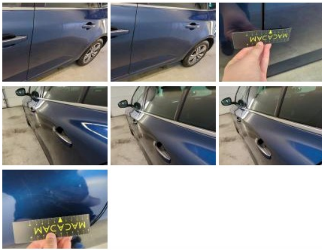
Outer sill L, Scratch(es), Repair and paint (complete)
