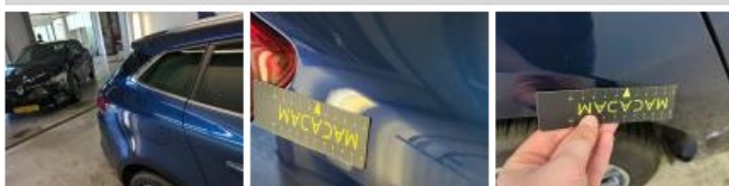
Door RR, Dent(s), Repair and paint (complete)
