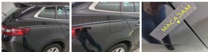
Door FR, Scratch(es), Repair and paint (complete)
