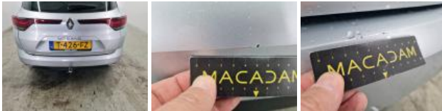
Bumper R, Scratch(es), Repair and paint (complete)
