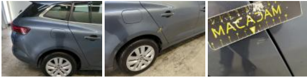
Door FR, Scratch(es), Repair and paint (complete)
