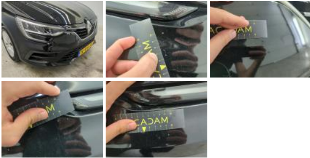
Door FR, Scratch(es), Repair and paint (complete)
