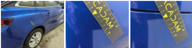
Door FR, Scratch(es), Repair and paint (complete)
