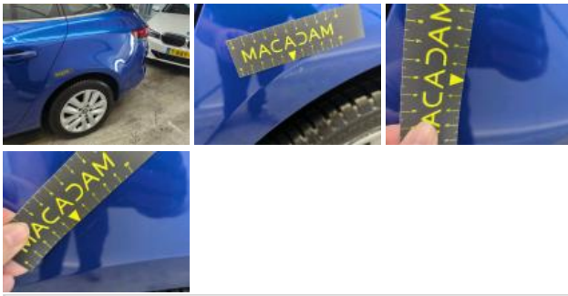
Door RL, Scratch(es), Repair and paint (complete)
