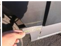
Outside rear-view mirror housing R, Scratch(es), Acceptable
