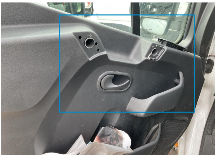
23. Interior door handle Front left Interior / Broken -
