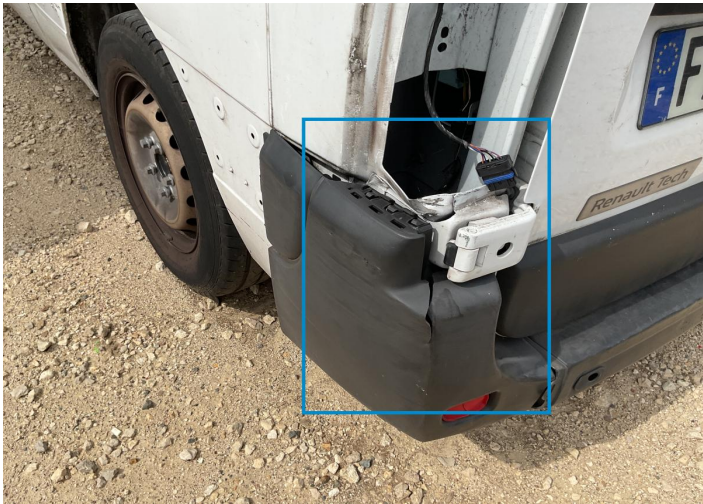
15. Bumper / Back Bodywork / Breakage / Hole -
