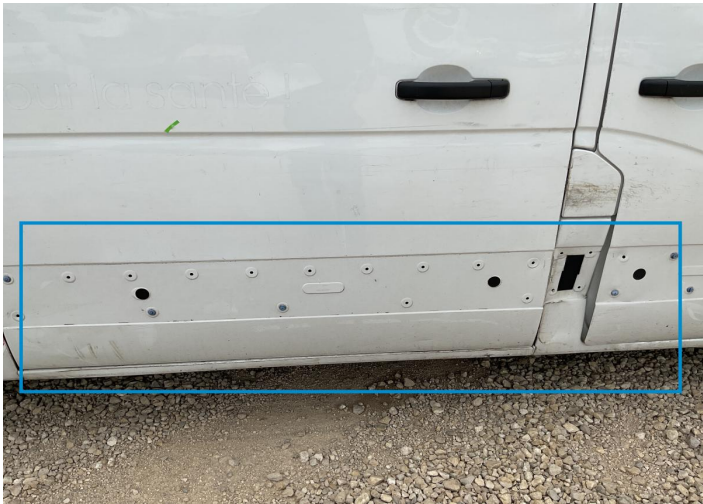
9. Door Side Molding / Front Right Bodywork / Breakage / Hole -
