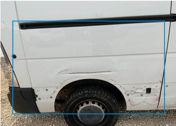
10. Side Panel / Back Right Bodywork / Dent / Dent -
