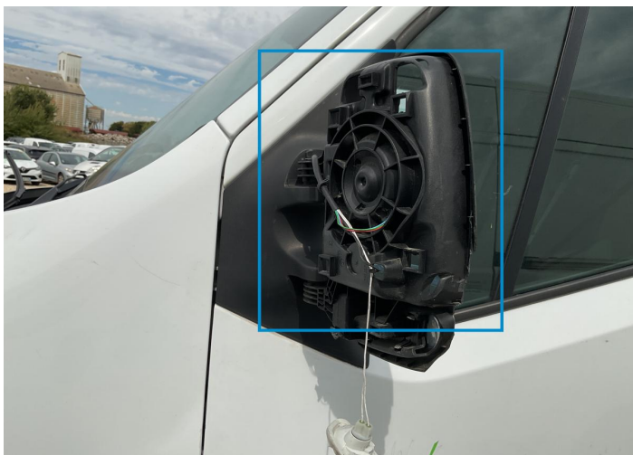
21. Mirror / Front Left Bodywork / Breakage / Hole -
