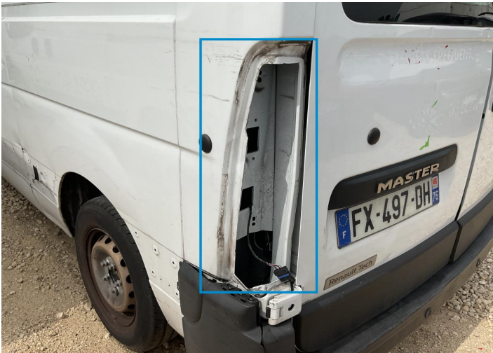
16. Tailgate Light / Back - Left Bodywork / Breakage / Hole -
