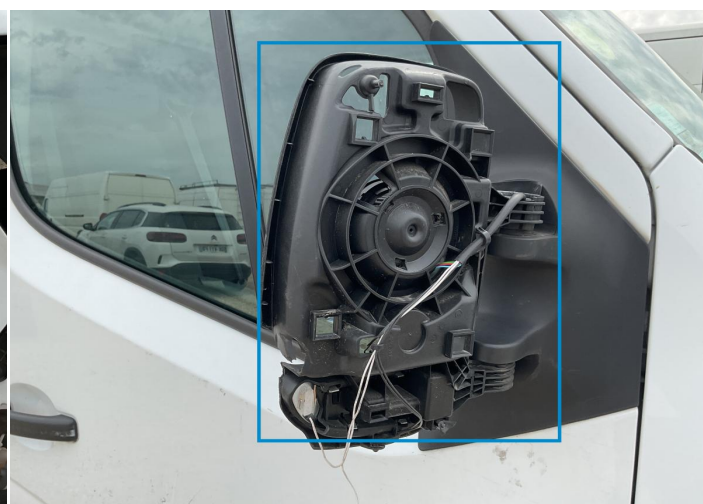
4. Mirror / Front Right Bodywork / Breakage / Hole -
