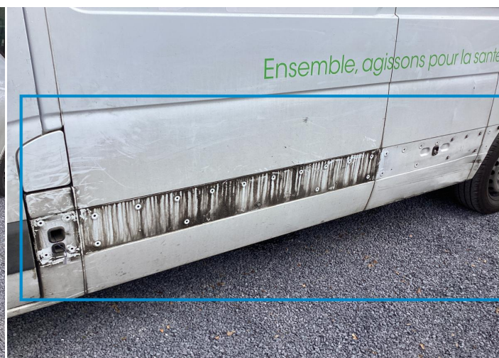
8. Rocker Panel / Center Left Missing Part -
