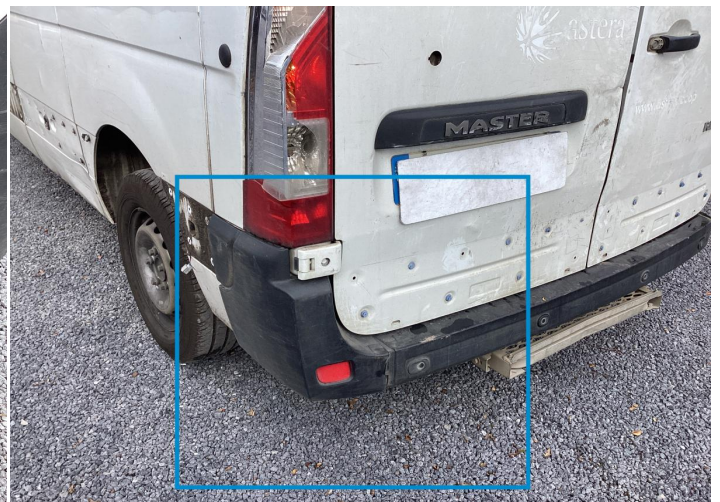
24. Corner Bumper / Back Left Paint / Scratch / Scuff -
