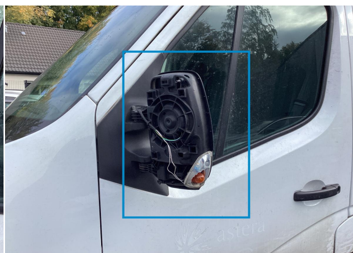
30. Mirror / Front Left Bodywork / Breakage -
