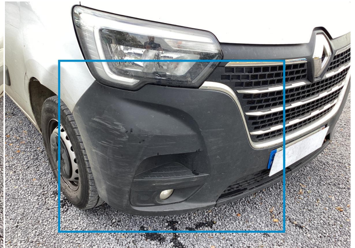
14. Corner Bumper / Front Right Paint / Scratch / Scuff -
