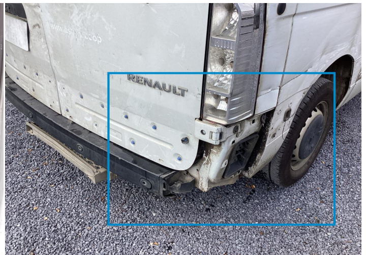
18. Corner Bumper / Back Right Missing Part -
