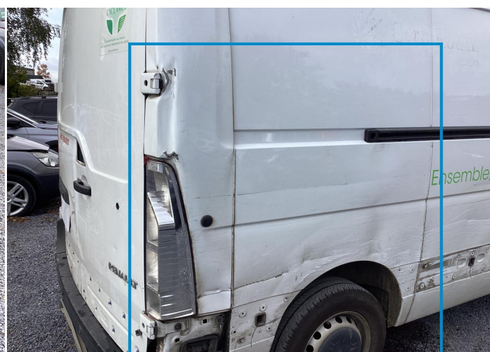
6. Side Panel / Back Right Bodywork / Dent / Deformation -
