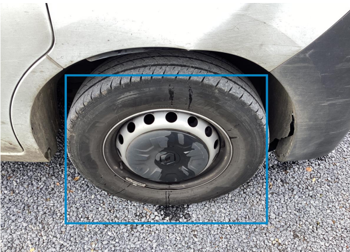
23. Rim / Front Right Out of Bodywork / Scratch -
