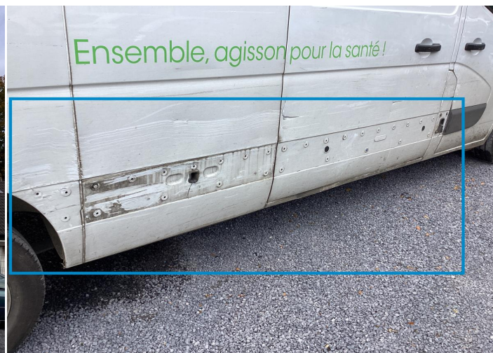
12. Rocker Panel / Center Right Missing Part -
