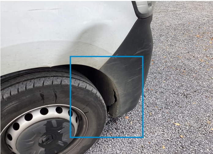
31. Mud Barrier / Front Right Bodywork / Breakage -
