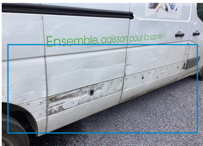
7. Side Panel / Back Right Paint / Scratch / Scuff -
