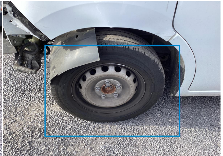
14. Rim / Front Left Out of Bodywork / Scratch -
