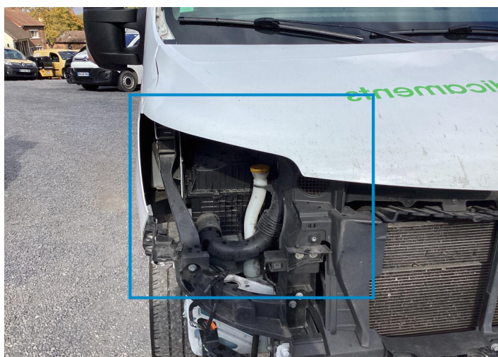
21. Front Light / Front Right Missing Part -
