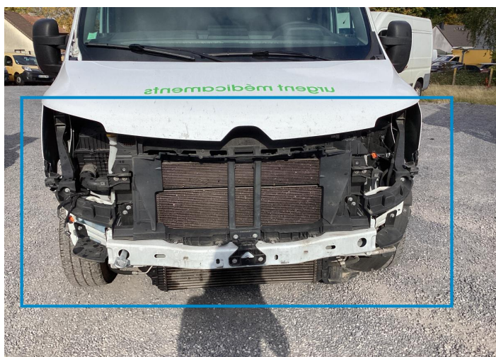
7. Bumper / Front Missing Part -
