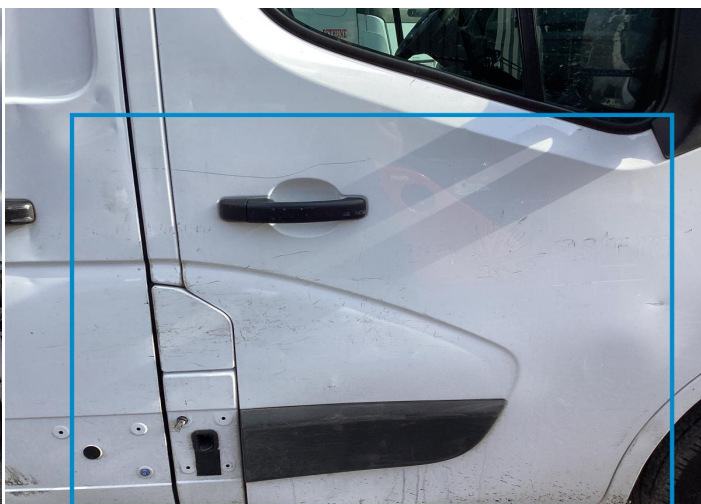
2. Door / Front Right Paint / Scratch / Scuff -
