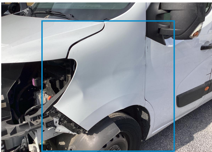
5. Fender / Front Left Bodywork / Dent / Deformation -
