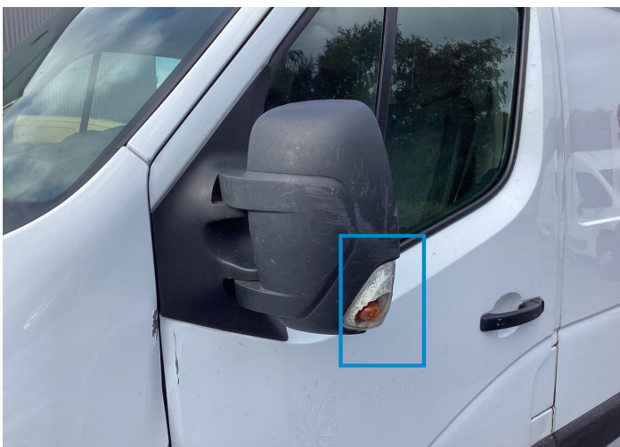
30. Mirror / Front Left Bodywork / Breakage -
