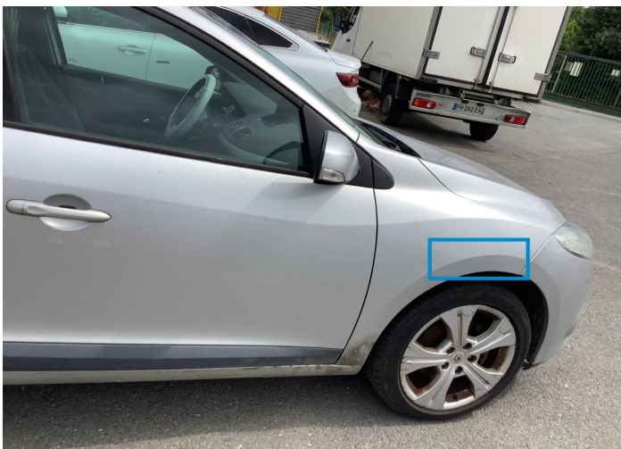
22. Fender / Front Right Paint / Scratch / Line -
