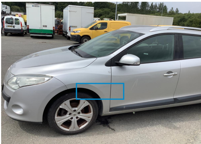
5. Fender / Front Left Paint / Stone Chip -
