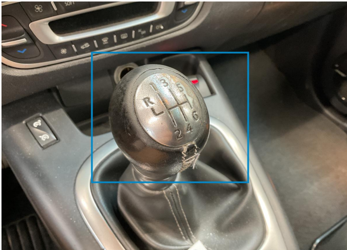
3. Gear Knob Interior / Broken -
