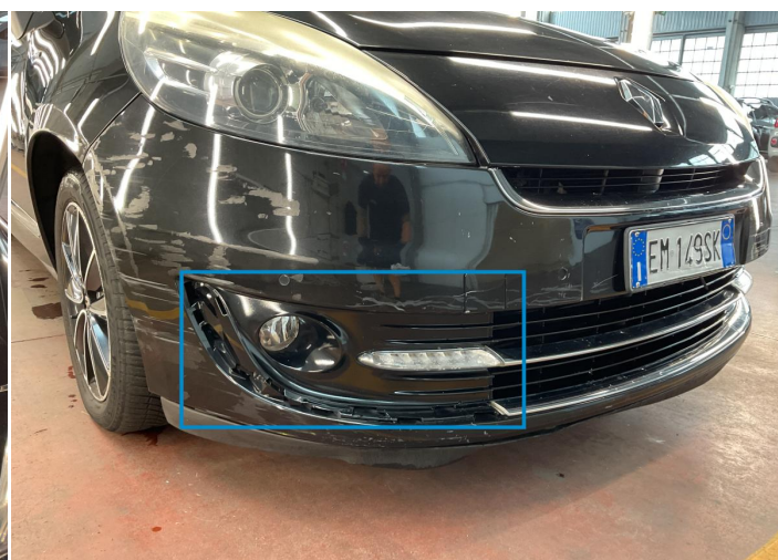
10. Bumper / Front Missing Part -
