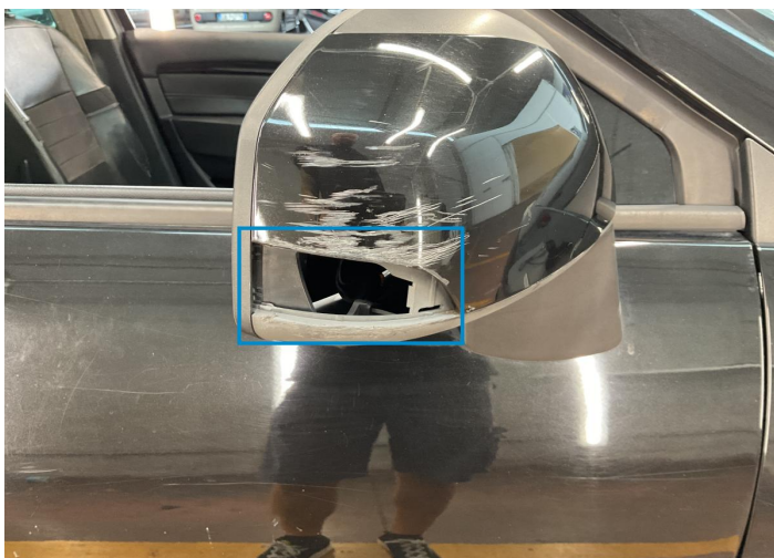
29. Mirror Repeater / Right Missing Part -
