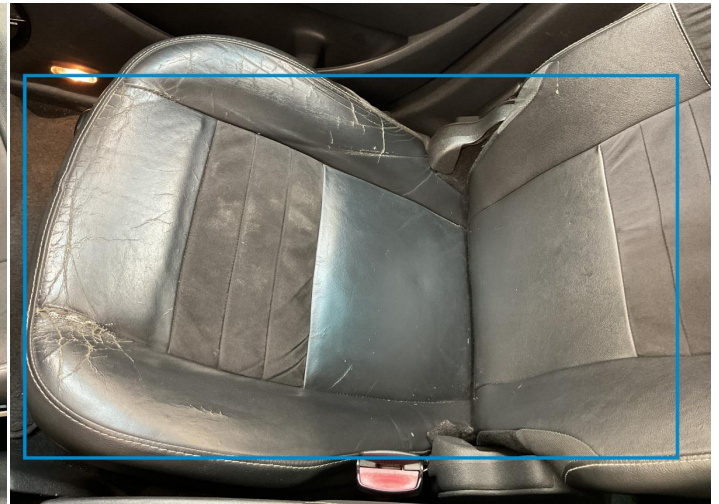
2. Seat / Front Right Interior / Ripped -
