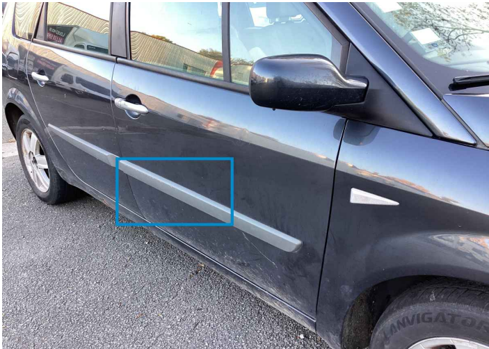
51. Door / Front Right Paint / Scratch / Line -
