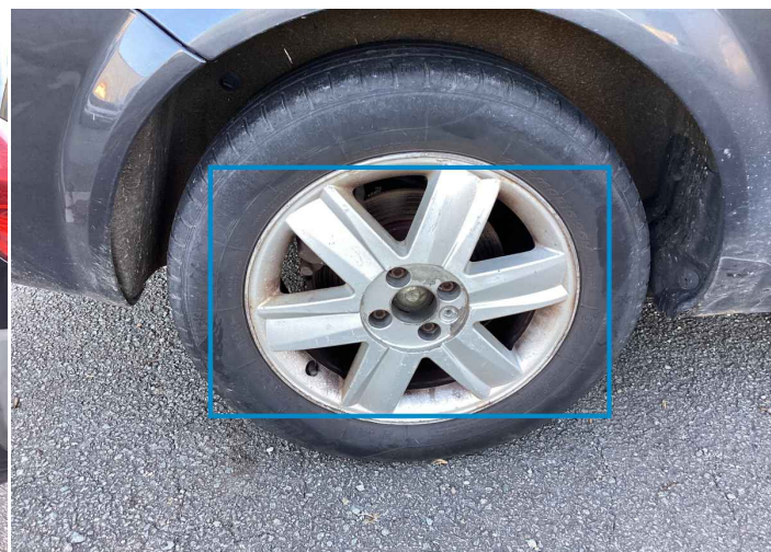
32. Rim / Back Right Out of Bodywork / Scratch -
