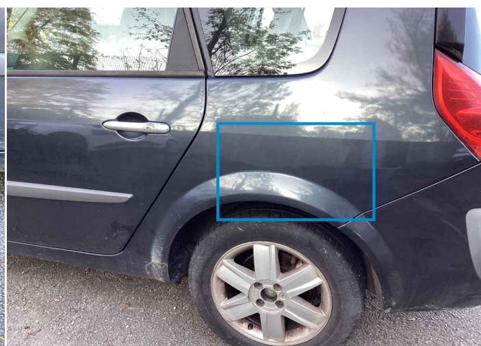
42. Side Panel / Back Left Paint / Chipping -
