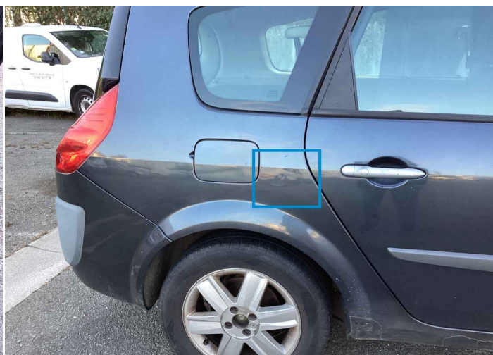
60. Side Panel / Back Right Bodywork / Dent / Deformation -
