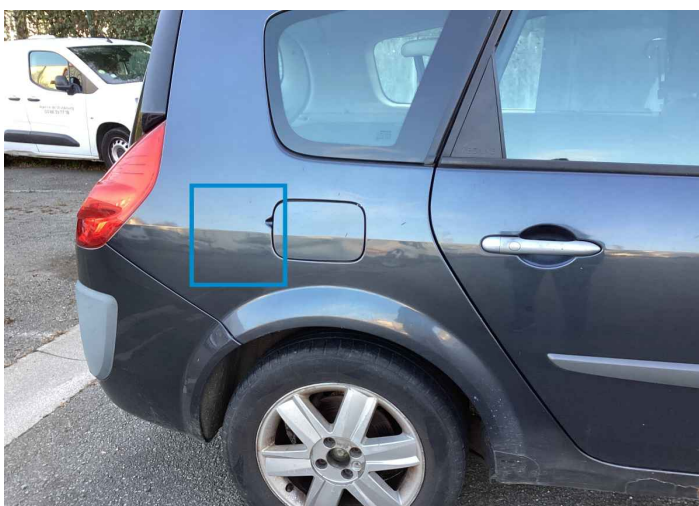
57. Side Panel / Back Right Bodywork / Dent / Deformation -
