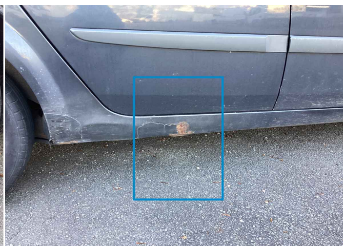
38. Rocker Panel / Center Right Paint / Corrosion -
