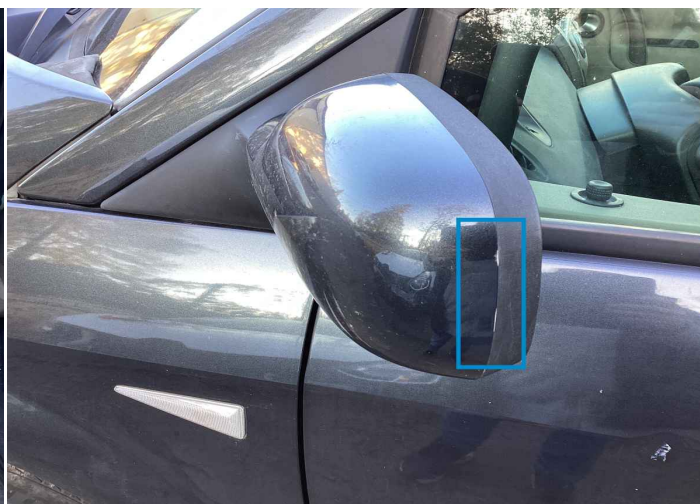
56. Mirror Shell / Front Left Paint / Scratch / Line -
