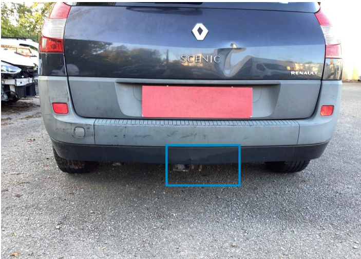
54. Bumper / Back Bodywork / Breakage -
