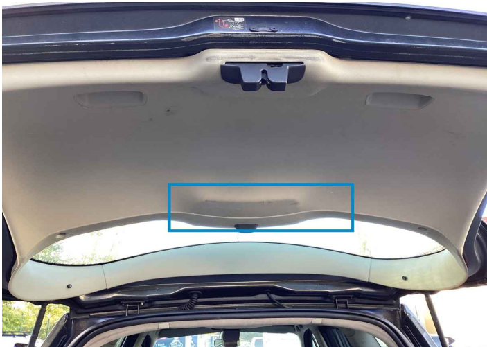
49. Trunk Upholstery / Back Interior / Scraped -
