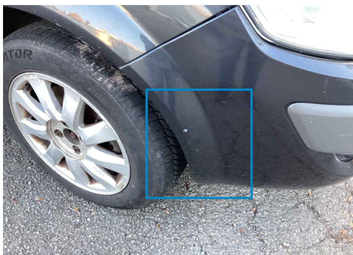
39. Corner Bumper / Front Right Paint / Chipping -
