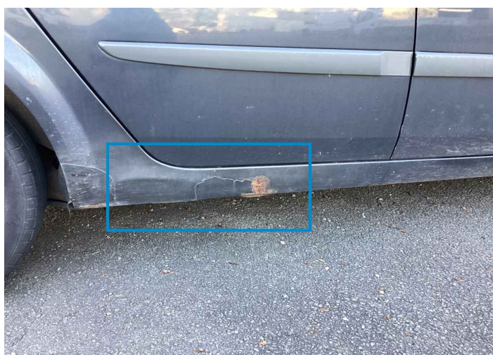
41. Rocker Panel / Center Right Bodywork / Dent / Deformation -
