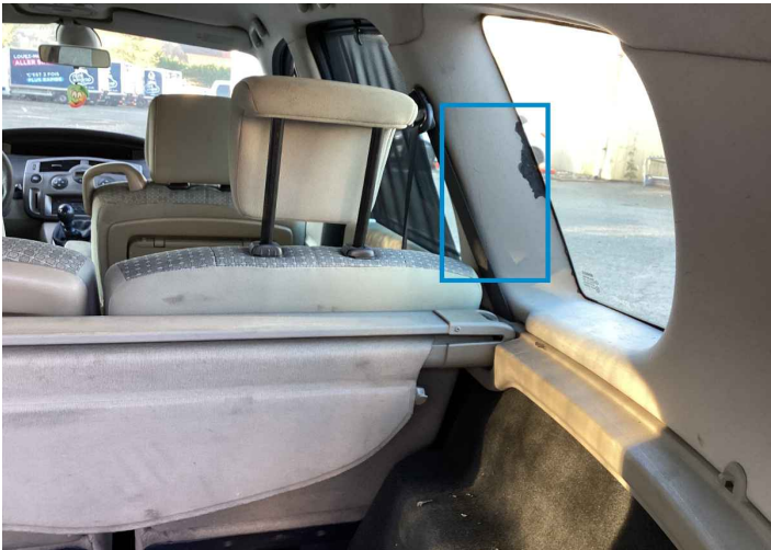
52. Trunk Upholstery / Back Interior / Scraped -
