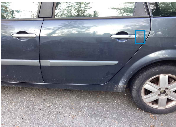
65. Door / Back Left Bodywork / Dent / Deformation -
