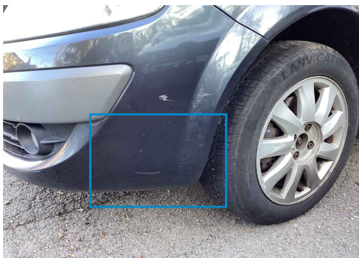
37. Corner Bumper / Front Left Paint / Scratch / Line -
