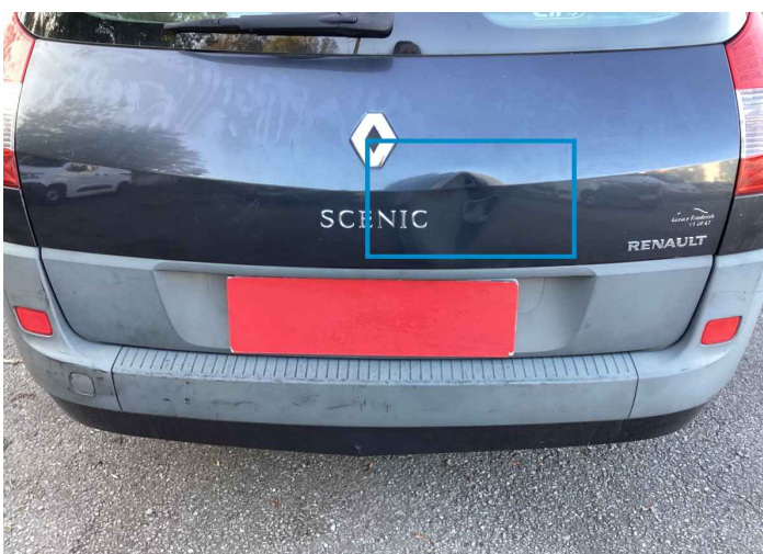
48. Tailgate Bodywork / Dent / Deformation -
