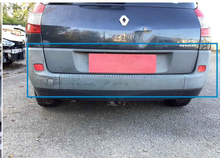
26. Bumper / Back Paint / Scratch / Line -
