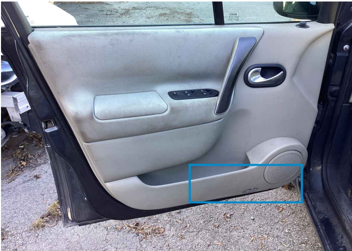
50. Panel Filling / Front Left Interior / Scraped -
