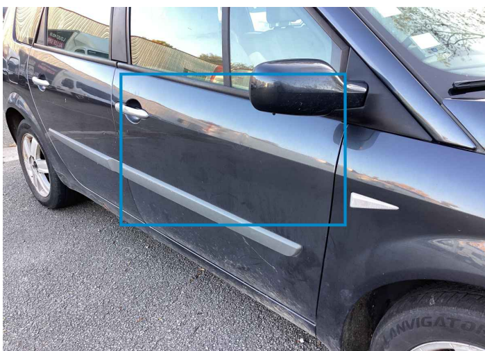
33. Door / Front Right Bodywork / Dent / Deformation -
