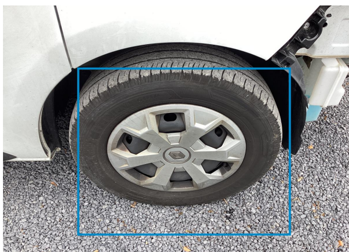
5. Hubcap / Front Right Out of Bodywork / Scratch -
