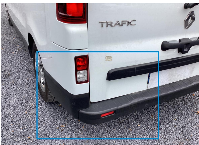
6. Corner Bumper / Back Left Paint / Scratch / Scuff -
