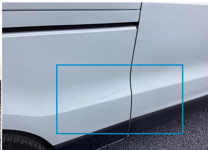
12. Door / Back Right Paint / Scratch / Line -
