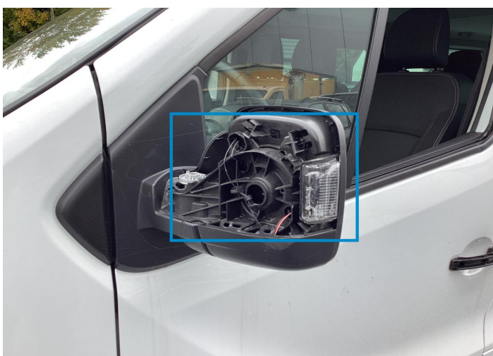
17. Mirror / Front Left Missing Part -
