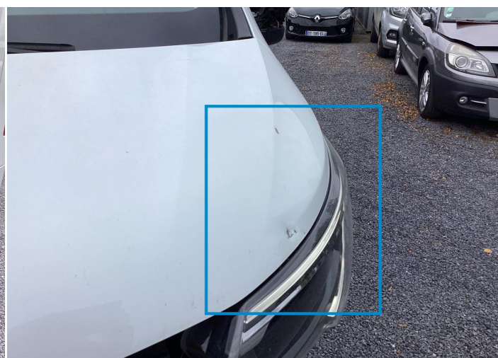
16. Hood Bodywork / Dent / Deformation -
