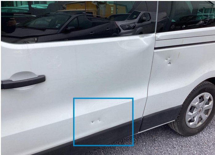
19. Door / Back Left Bodywork / Dent / Deformation -
